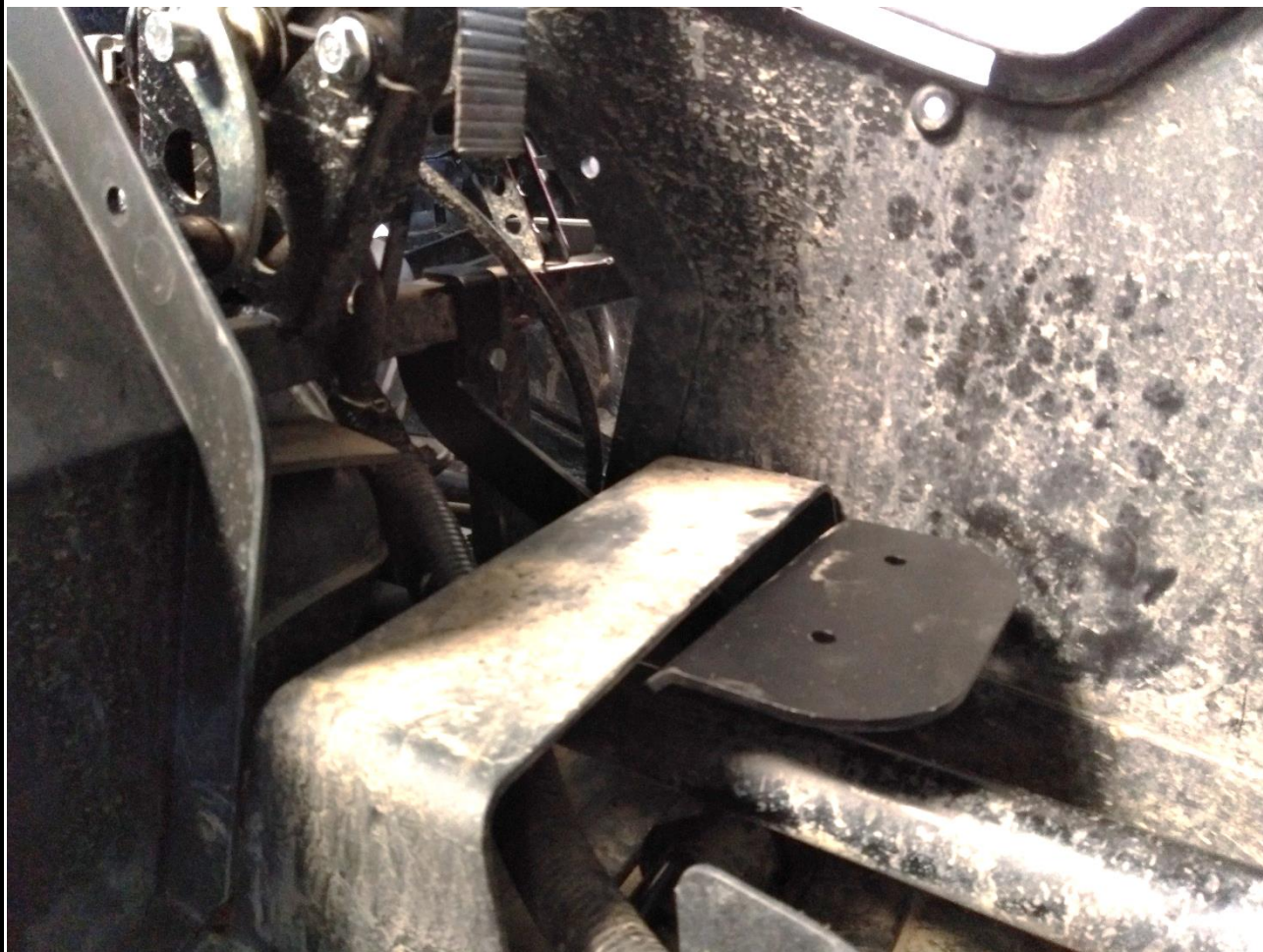
Photo of mounted heater holder.
