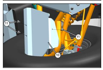
Install the rear A-arm guards (9,10) to the rear A-arms using screws (11). Torque the fasteners to specification.
