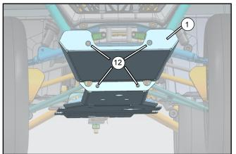
// Install the winch armor (1) to the corresponding position, connect the front skid plate, and tighten it with screws (12). Torque the fasteners of the rear, center, and front skid plates to specification.
