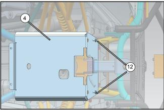
Install the rear skid plate (4) to the corresponding position at the bottom of the vehicle with screws (12) and finger-tighten.
