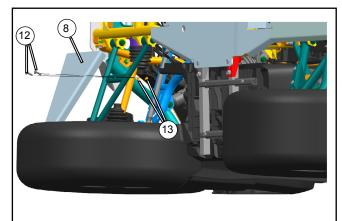
Install the front A-arm guards (7,8) to the front A-arms using the screws (12) and nuts (13). Torque the fasteners to specification.
