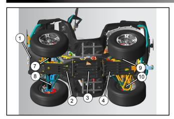
Remove the existing winch armor (1), left and right front A-arm guards (7)(8), front skid plate (2), center skid plate (3), rear skid plate (4), left and right rear A-arm guards (9)(10).
